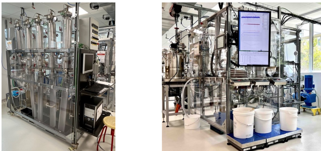
Figure 2. PHUN-0 (left) Subcritical water hydrolysis pilot plant in cycles and PHUN-2 (right) Supercritical water hydrolysis pilot plant in continuous
