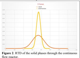
Baffles were placed in the reactor to ensure plug flow in the continuous reactor, and the RTD of both liquid and solid phases were measured, with results as shown in Figure 2. The RTD of the liquid phase is showed substantial departure from plug flow, with a dispersion number of 0.0219. This may reflect laminar flow conditions of the reactor. The particles, however, were nearly in plug flow, with a dispersion number of 0.0029.
