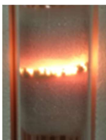
Figure 1. Ignited bed in 7.5 mm lab reactor
