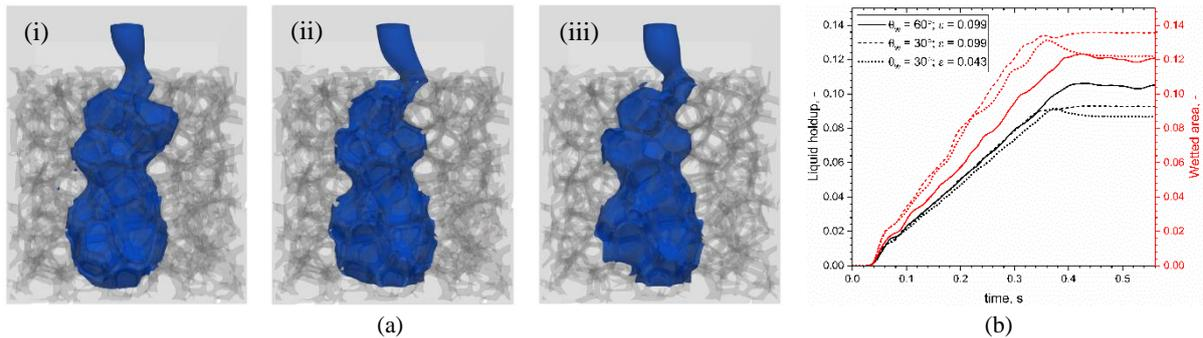
**Figure 2.** (a) Steady-state local liquid distribution at (i)  $\varepsilon = 0.099$ ,  $\theta_w = 60$ ; (ii)  $\varepsilon = 0.099$ ,  $\theta_w = 30$ ; (iii)  $\varepsilon = 0.043$ ,  $\theta_w = 30$  (note: water and foam is colored blue and grey, respectively. Air is transparent) and (b) effect of  $\varepsilon$  as well as  $\theta_w$  on normalized liquid holdup and wetted area (10 pore/inch,  $V_L = 0.11$  m/s,  $V_G = 0.167$  m/s).
