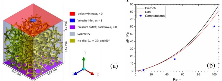
**Figure 1.** (a) Computational domain of open-cell foam along with boundary conditions and (b) single-phase pressure drop predictions compared with semi-empirical correlations ( $\varepsilon = 0.043, 10$  pores/inch).
