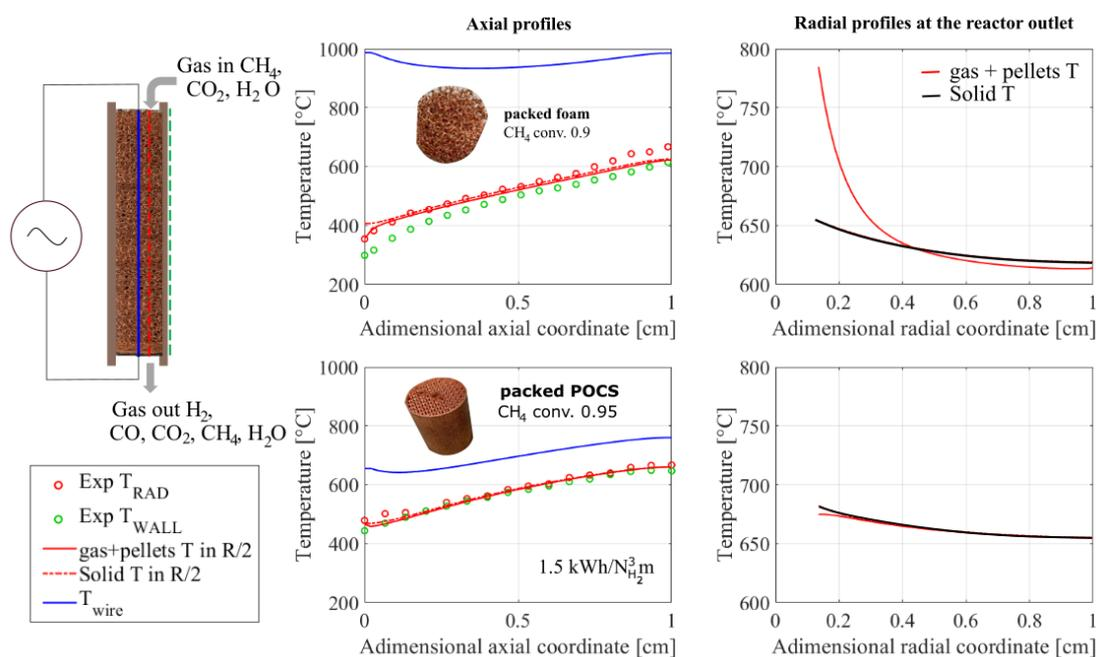
**Figure 1.** Scheme of the lab-scale electrified reactor with the temperature profiles obtained for packed foams and packed POCS in steam biogas reforming experimental (dots) and according to model simulations (lines).
