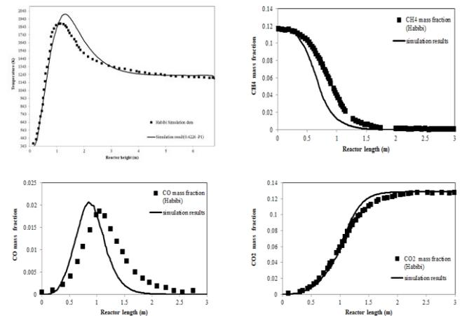
**Figure 2.** Static temperature and the species concentration for the right hand side burner across the height of the furnace.
