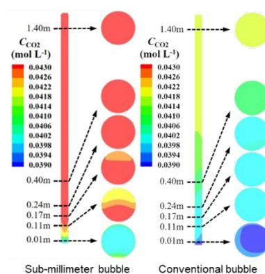
**Figure 2.** Comparison of  $\text{CO}_2$  concentration distribution in Laboratory-scale bubble column.
