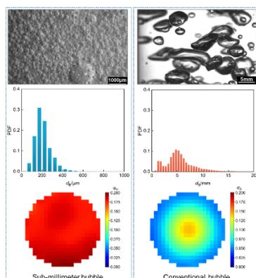
**Figure 1.** Comparison of bubble size distribution and gas holdup distribution.
