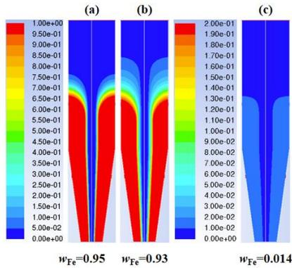
**Figure 1.** Metallization rate under rate constants from Tsay et al (a), Takahashi et al (b), and Hamadeh et al (c).
