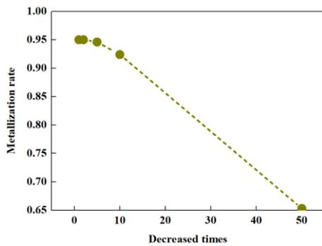
**Figure 3.** Product metallization rate with decreased times of gas diffusivity in pellets.
