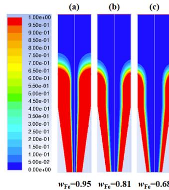
**Figure 2.** Metallization rate against bed permeability: base case (a), decreasing 1.67 (b) and 2.86 (c) times.
