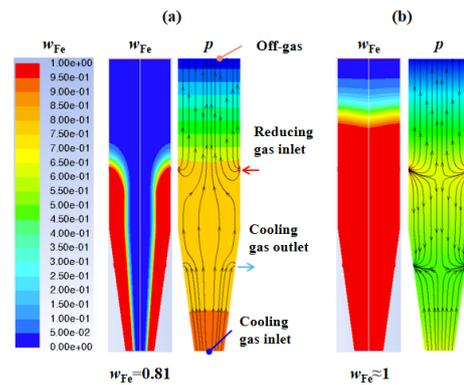
**Figure 4.** Metallization rate and flow field: base case (a) and improved case (b).
