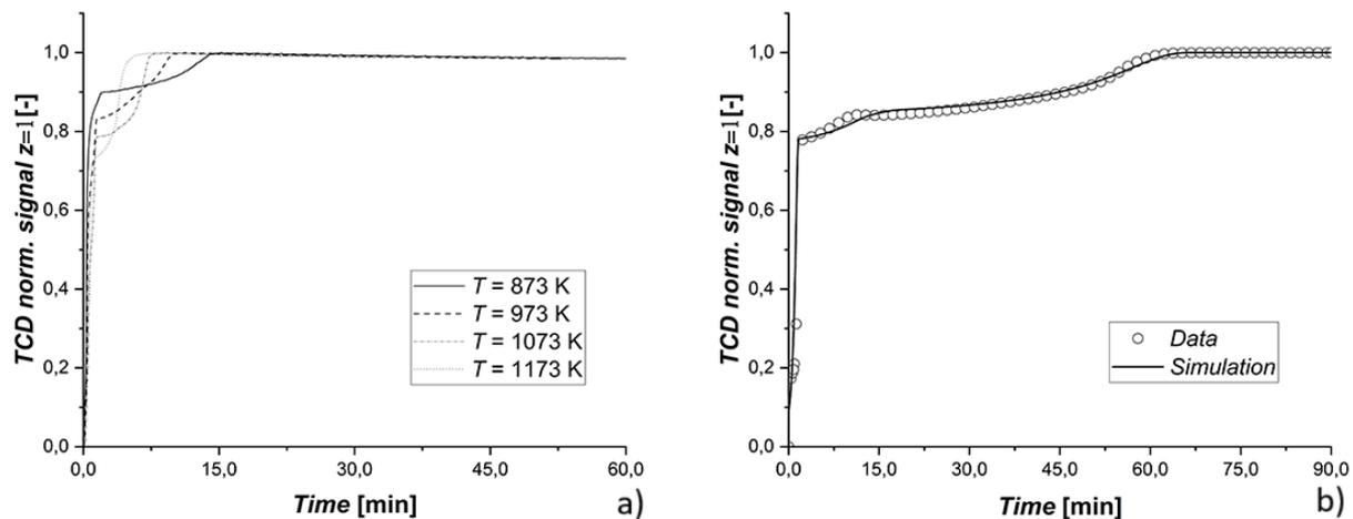
Figure 1. a) Examples of experimental results on the reduction of a monolayer of hematite powder at different operating temperatures, b) Preliminary comparison between bed experimental data and simulation.
