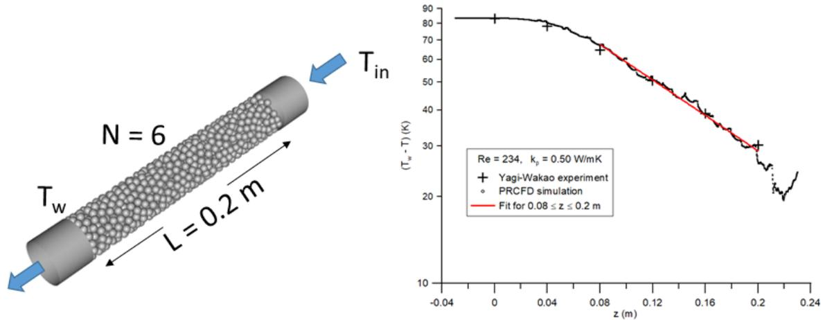
**Figure 1.** Isometric view of simulated fixed bed (left); fit of straight line to PRCFD axial temperatures (right).
