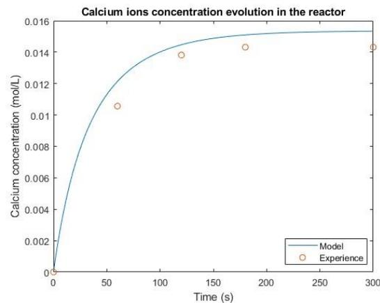
**Figure 2.** Model experiment comparison after transfer coefficient estimation for concrete particle dissolution with diameters of 0 to 250  $\mu\text{m}$ , an initial pH of 2, a solid concentration of 25g/L at room temperature
