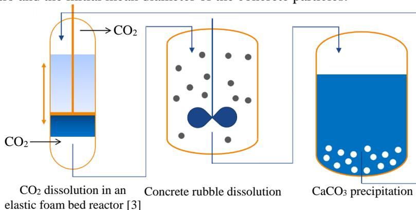
**Figure 1.** Example of succession of the three main unit operations
