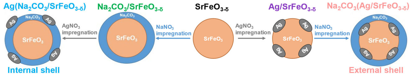
Figure 1. Schematic showing summary of samples prepared by sequential impregnation with Ag and \text{Na}_2\text{CO}_3
