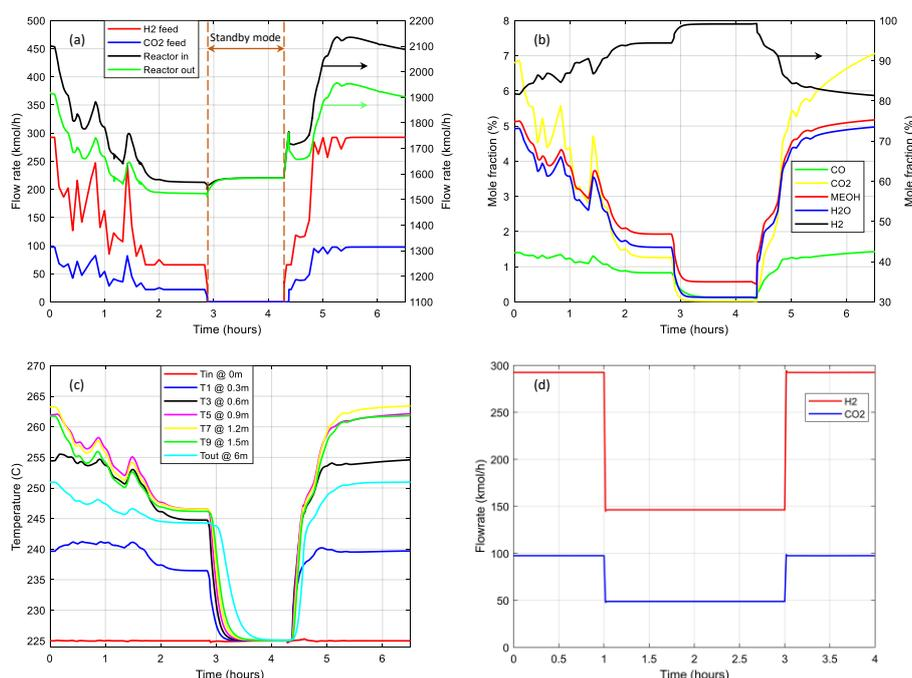
**Figure 2.** (a) Flowrate of feeds and the reactor streams; (b) reactor outlet composition; (c) reactor temperature along the length under variation of H<sub>2</sub>; (d) Maximum achievable ramping rates of the model between 100 % ↔ 50 % load.
